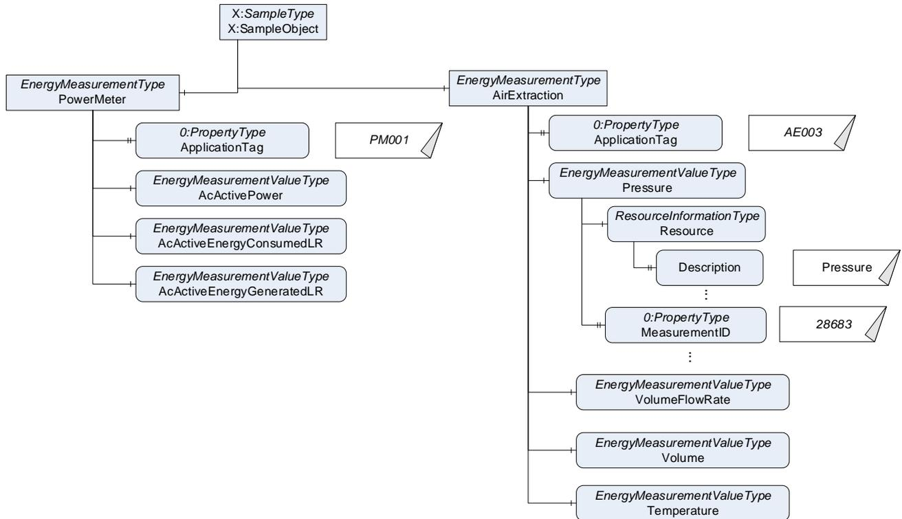
**Figure 9 – Example of usage of EnergyMeasurementType**
