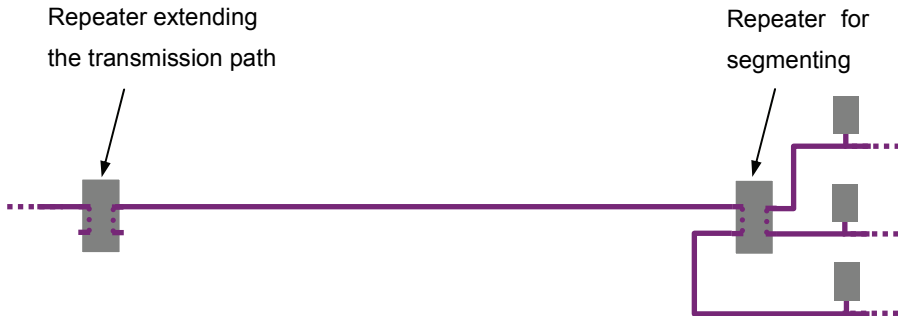
Figure 2-7 Possible application of repeaters
