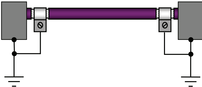
Figure 3-29 Standard grounding concept for PROFIBUS
