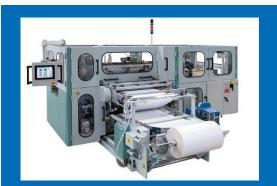
The use of PROFIBUS with the PROFIdrive profile is widespread in the control of packaging machines. All functions are executed on a single bus, which considerably reduces the expenditure for engineering, hardware and training.
