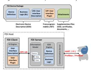
Fig. 19: FDI Device Package and FDI host
