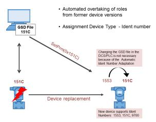
Fig. 12: Device replacement with transfer of the predecessors' functions
