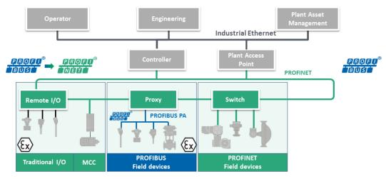
Fig. 25: PROFINET in the field with PROFIBUS PA integrated via a proxy
