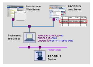
Fig. 16: The principle of I&M functions
