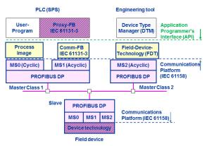
Fig. 11: The use of function blocks (Proxy FB and Comm FB)
