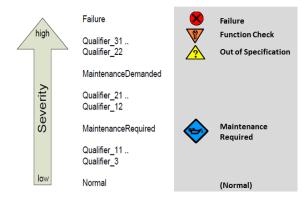
Fig. 26: Assignment of the PROFINET device diagnostics to NE 107
