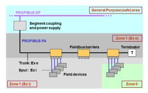
Fig. 5: Utilization of different ignition protection types
