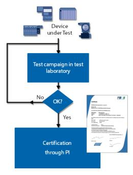
Fig. 23: Device certification, test procedure
