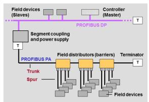
Fig. 6: The connection of DP and PA segments
