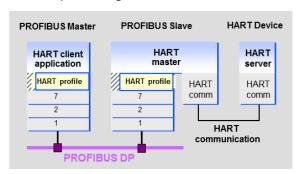
Fig. 15: Operating HART devices on PROFIBUS
