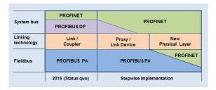
Fig. 24: Stepwise introduction of PROFINET in the intrinsically safe field
