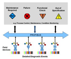
Fig. 14: Diagnostic mapping as per NAMUR recommendation 107
