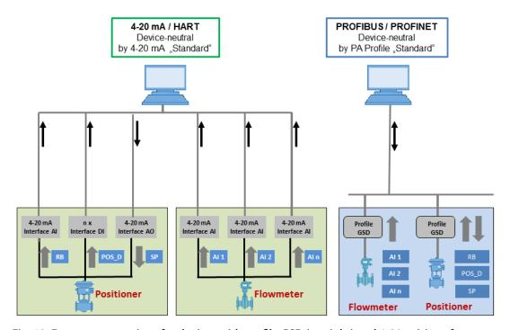
Fig. 18: Expense comparison for devices with profile GSD (on right) and 4-20 mA interface (on left)
