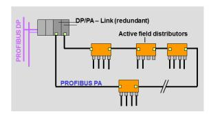
Fig. 8: Ring redundancy with PROFIBUS PA
