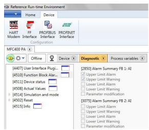
Fig. 20: EDD-based part of an FDI Device Package in the FDI reference host
