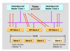
Fig. 10: Cyclical and acyclical communication with DP-V1
